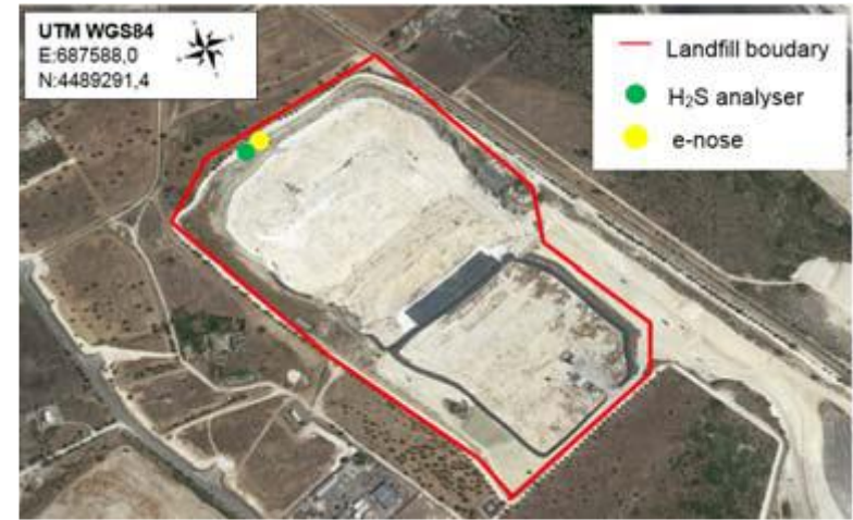
Figure 1b: sanitary landfill and monitoring points
